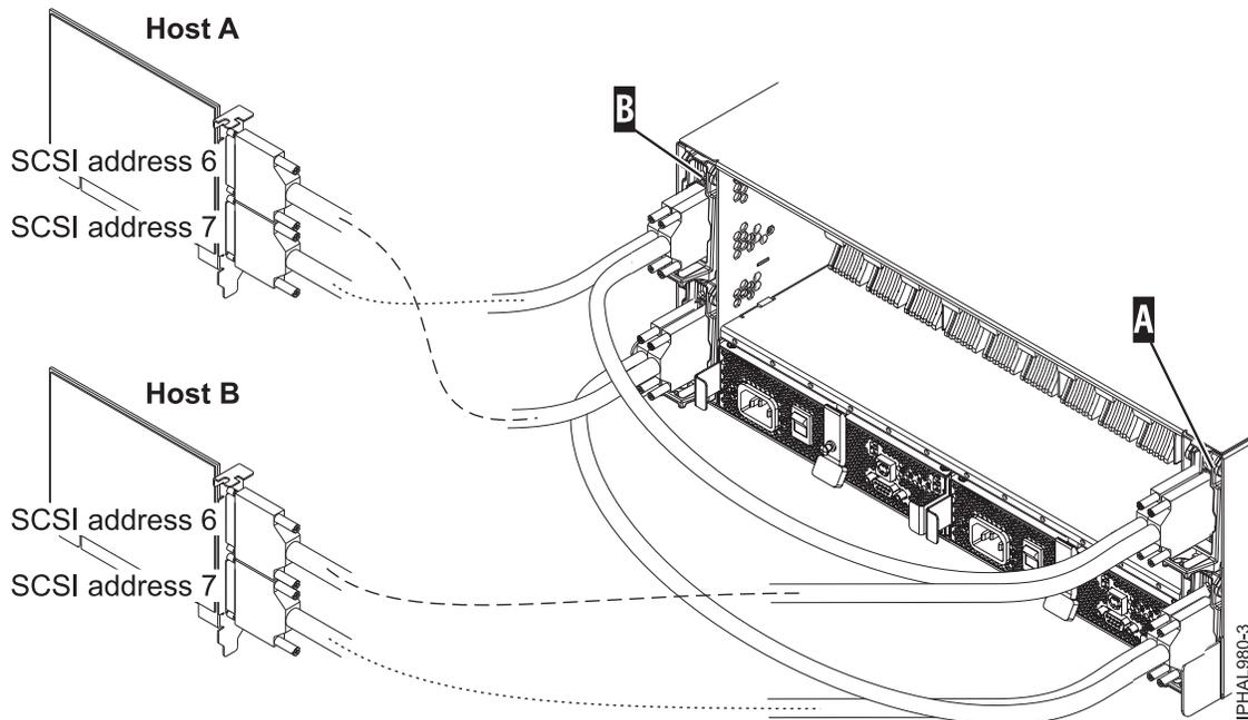
Figure 20. SCSI cable to dual repeater card connected with two SCSI cards
