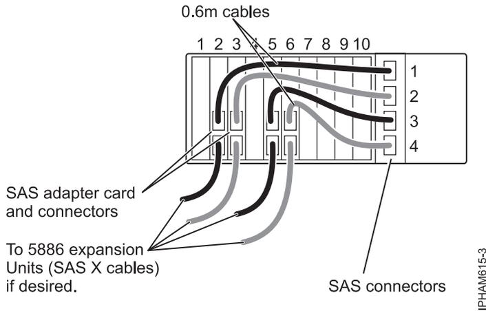
Figure 43. Physical cabling example: Two hard disk drive partitions with nine disks per hard disk drive partition, four SAS adapters, hard disk drive partitions switch position 2
