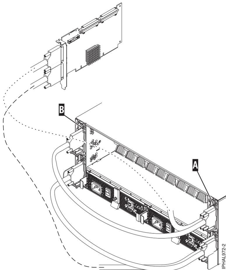
Figure 30. SCSI cable to a dual repeater card connected to a single repeater card
