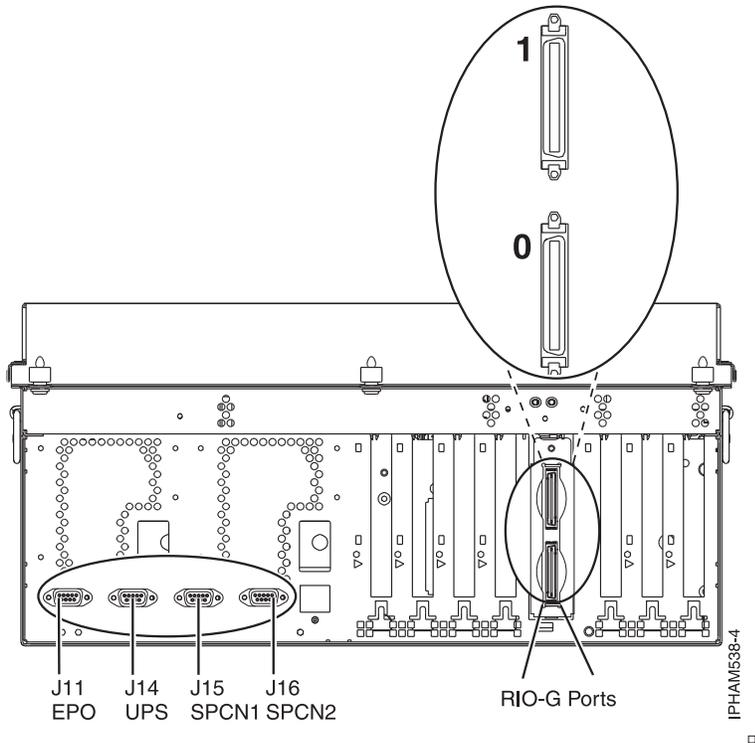
Figure 13. Model 0595 connector locations on rack-mounted unit
