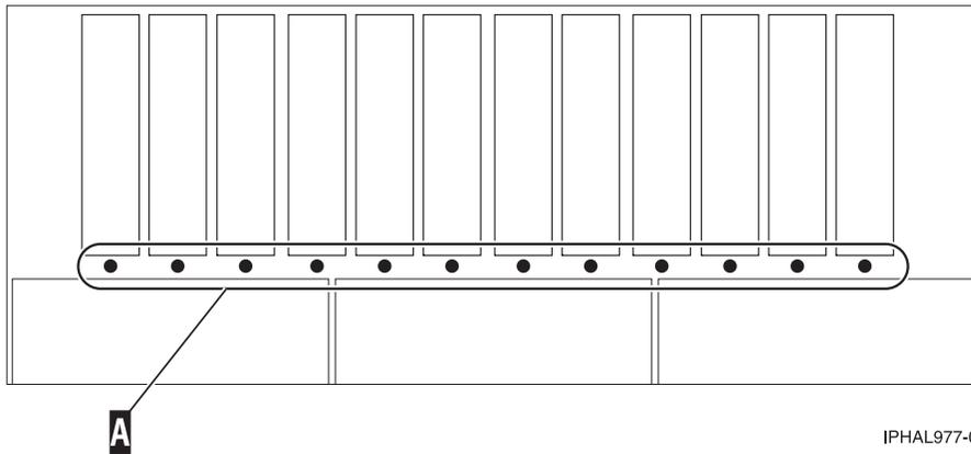
Figure 37. Front view of SCSI disk-drive enclosure concurrent maintenance lights for model 5786, 5787, 7031-D24, and 7031-T24
