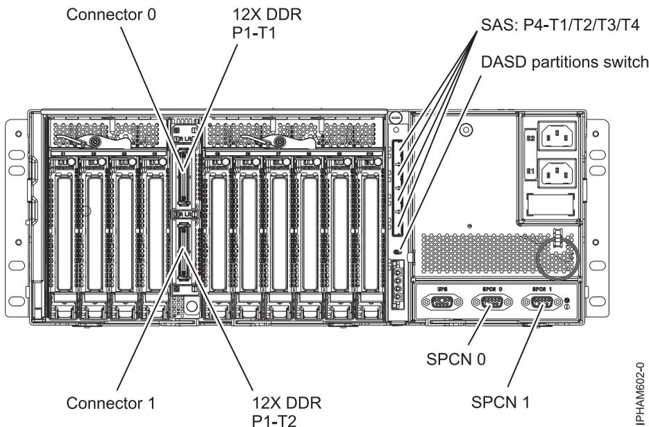
Figure 16. Model 5802 and 5877 connector locations
