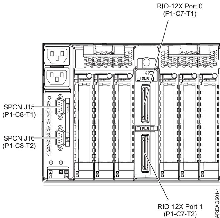
Figure 11. Model 5796 or 7314-G30 connector locations
