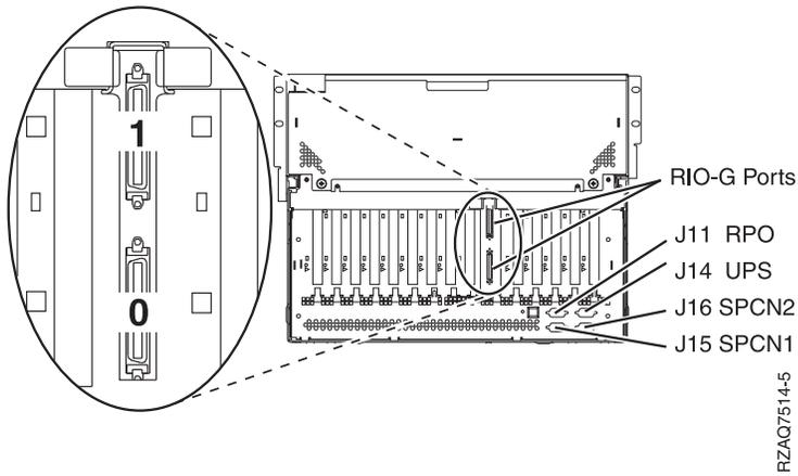
Figure 12. Model 0588 or 5088 connector locations
