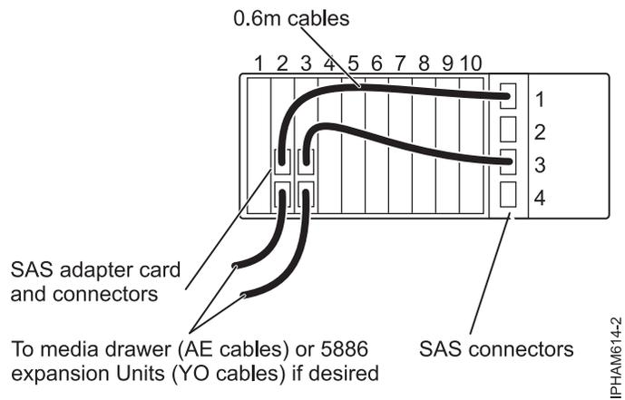
Figure 42. Physical cabling example: Two hard disk drive partitions with nine disks per hard disk drive partition, two SAS adapters, hard disk drive partitions switch position 2
