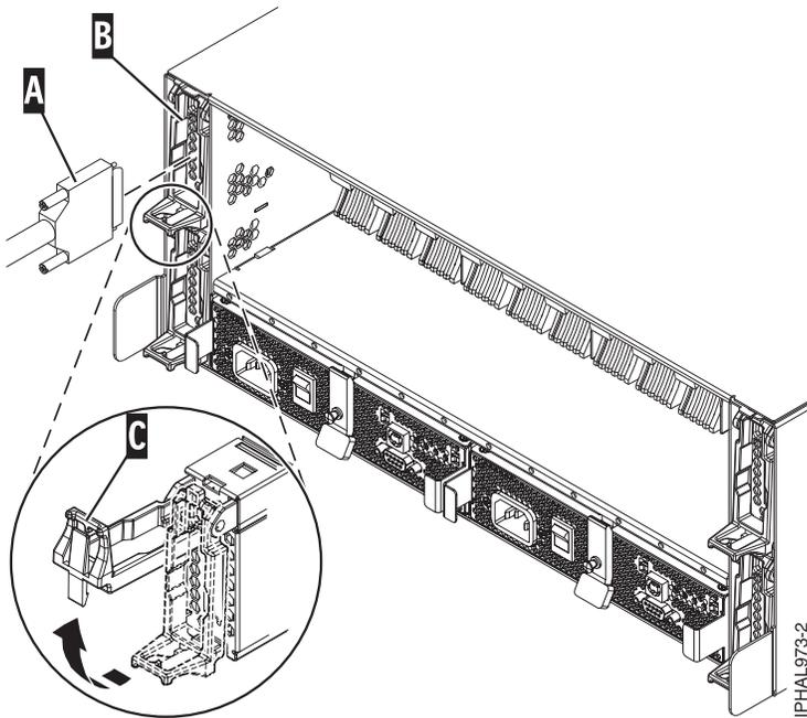
Figure 19. SCSI cable to single repeater card
