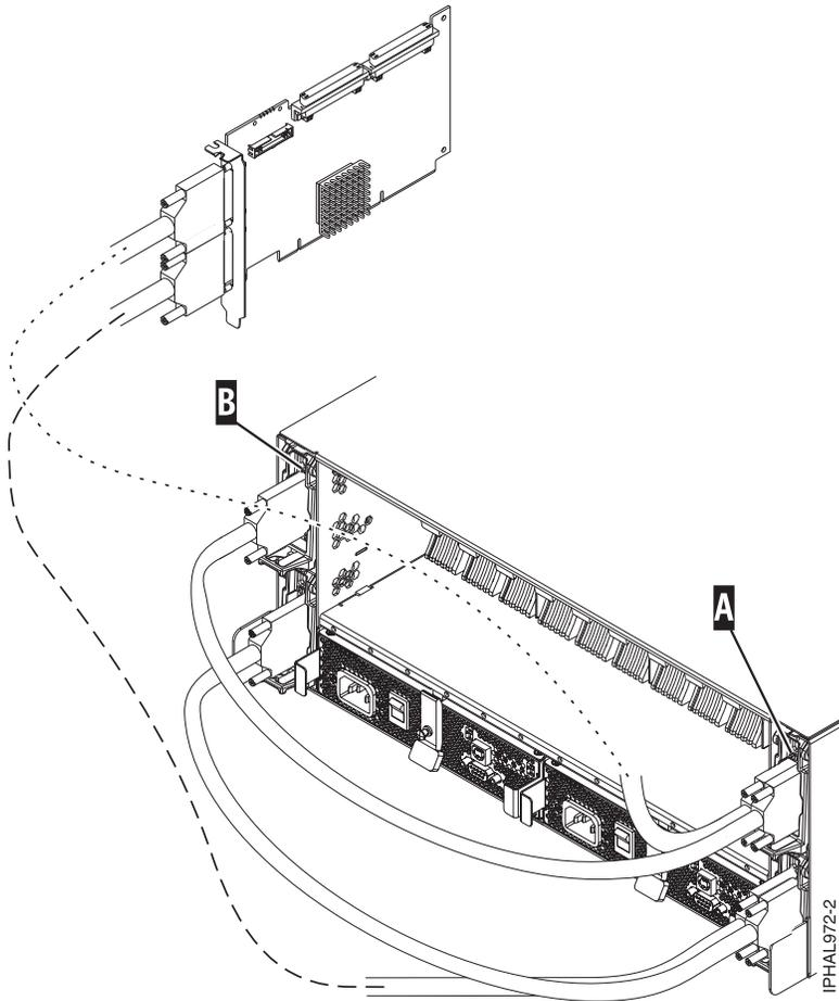
Figure 27. SCSI cable to a dual repeater card that is connected to a single repeater card
