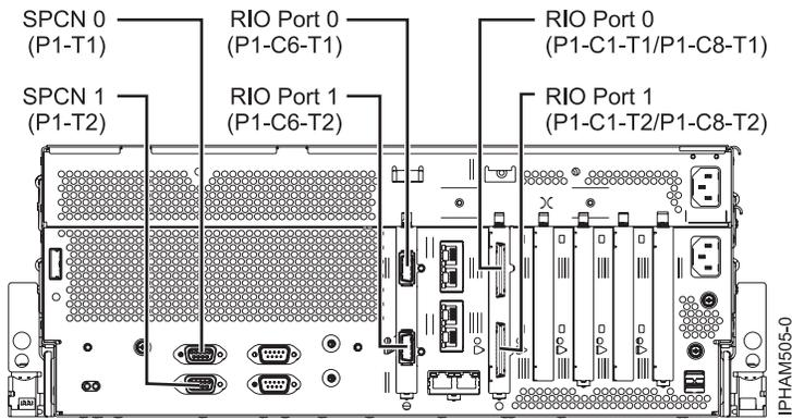
Figure 4. Model 8203-E4A, 8261-E4S, 9407-M15, and 9408-M25 connector locations on rack-mounted model
