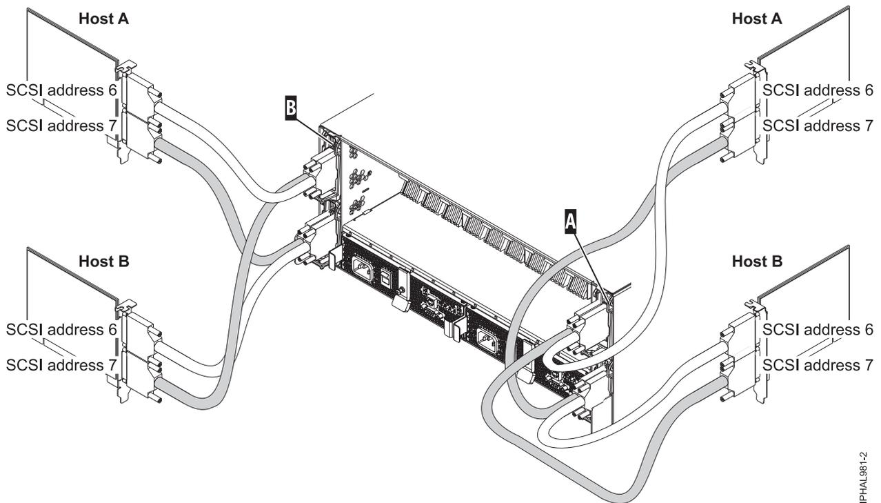
Figure 21. SCSI cable to dual repeater card connected with four SCSI cards
