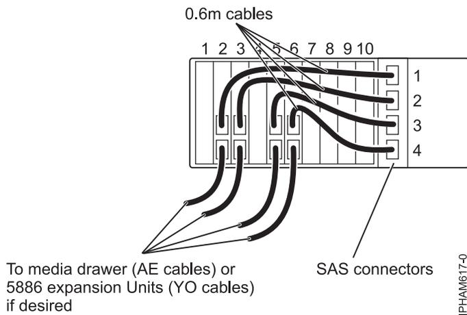
Figure 45. Physical cabling example: Four hard disk drive partitions with four or five disks per hard disk drive partition, hard disk drive partitions switch position 4
