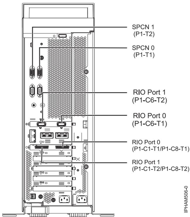
Figure 5. Model 8203-E4A, 8261-E4S, 9407-M15, and 9408-M25 connector locations on a stand-alone model
