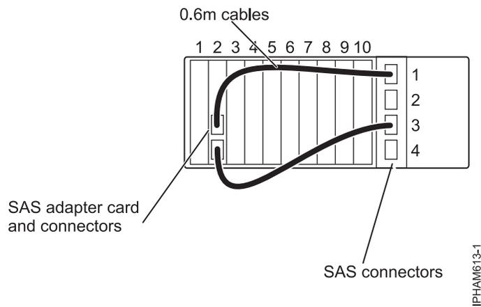
Figure 41. Physical cabling example: Two hard disk drive partitions with nine disks per hard disk drive partition, a single SAS adapter, hard disk drive partitions switch position 2
