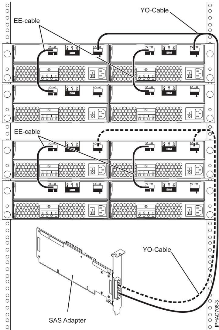
Figure 47. SAS YO cable to single enclosure with EE cables adding an additional enclosure or two YO connected enclosures each with an additional enclosure attached
