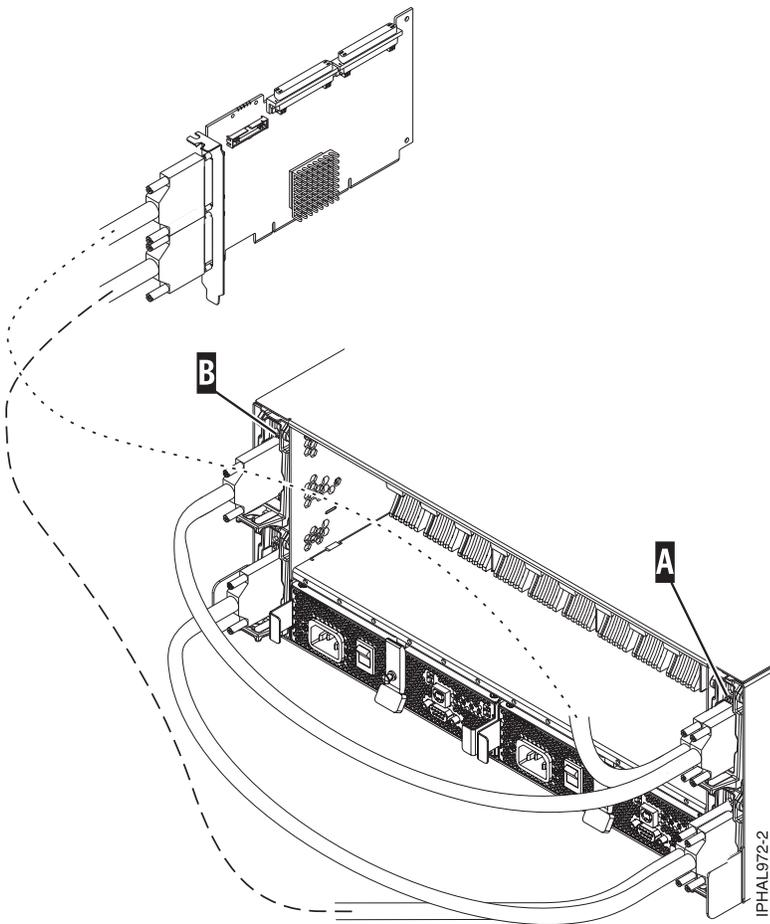
Figure 22. SCSI cable to dual repeater card connected to single repeater card
