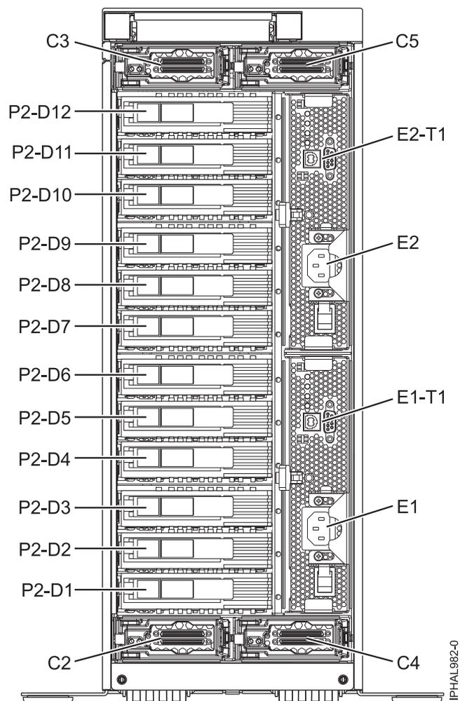
Figure 33. Repeater card location of the 5787 and 7031-T24 SCSI disk-drive enclosure (deskside models)
