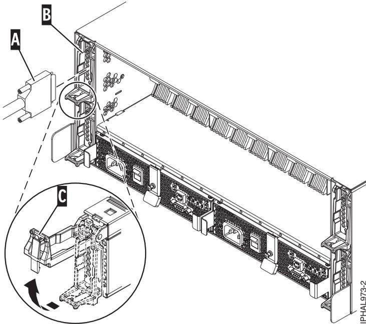
Figure 36. Removing SCSI cable from the repeater card
