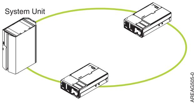
Figure 1. RIO/HSL, 12X, or 12X DDR loop example
