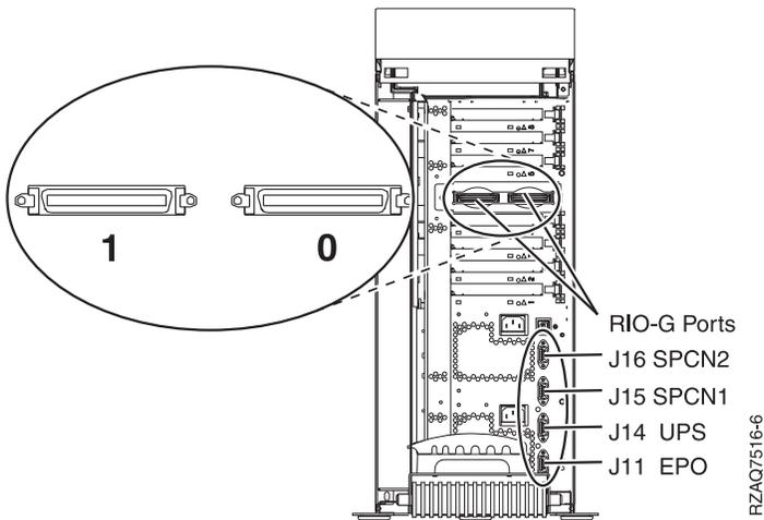
Figure 14. Model 5095 connector locations on stand-alone unit
