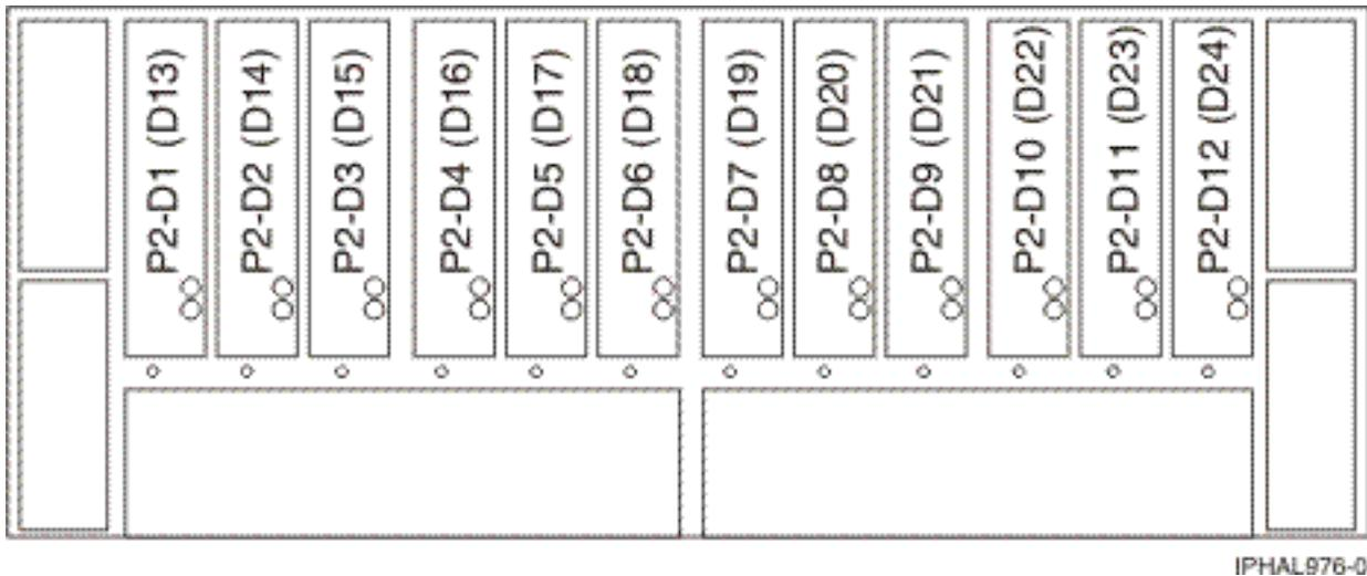
Figure 35. Back view of 5786, 5787, 7031-D24, or 7031-T24 SCSI disk-drive enclosure
