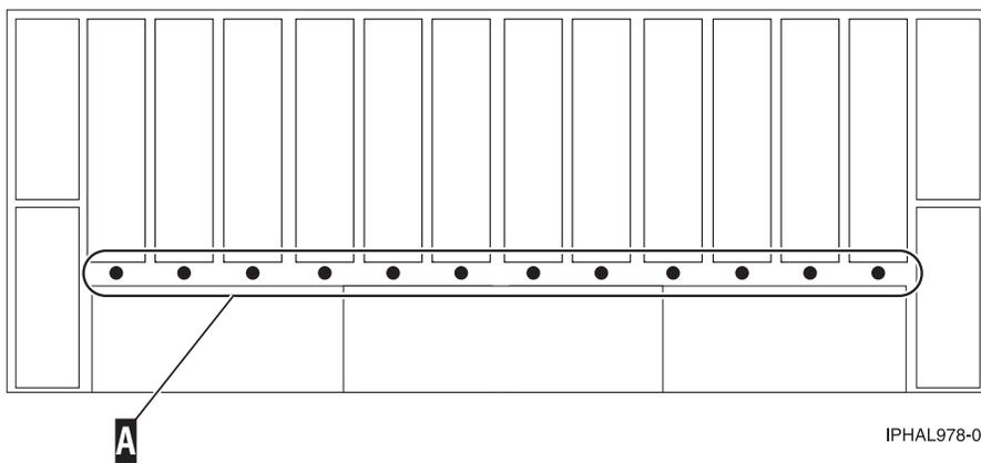
Figure 38. Back view of SCSI disk-drive enclosure concurrent maintenance lights for model 5786, 5787, 7031-D24, and 7031-T24
