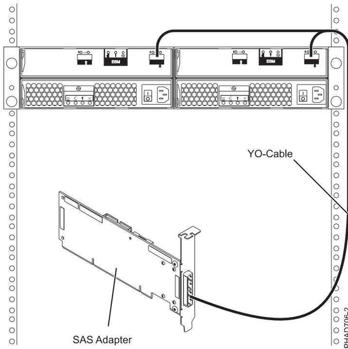
Figure 46. SAS YO cable to single enclosure card
