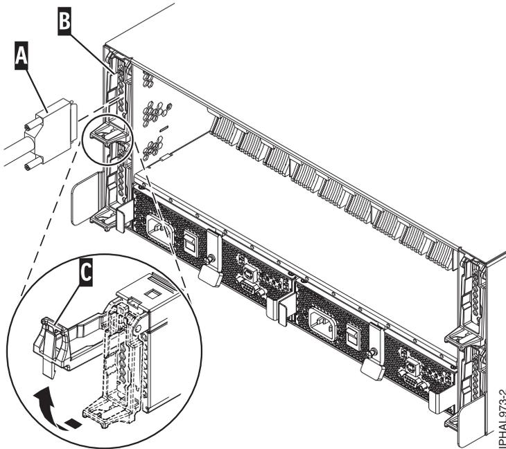
Figure 29. SCSI cable to a single repeater card
