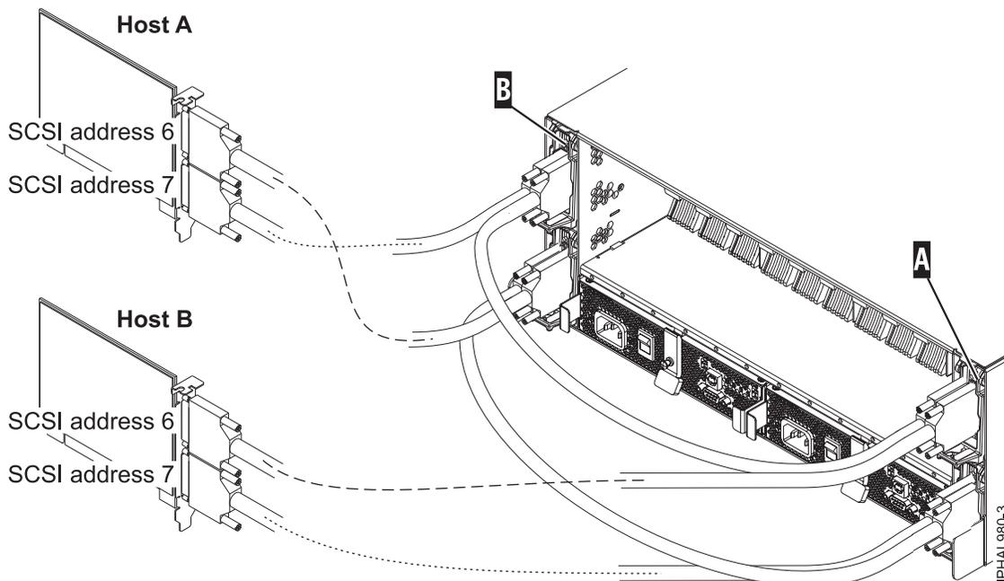
Figure 23. SCSI cable to a dual repeater card that is connected with two SCSI cards
