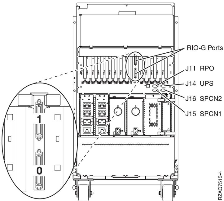
Figure 15. Model 5094, 5294, 5096, or 5296 connector locations
