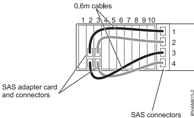
Figure 39. Physical cabling example: Two hard disk drive partitions with nine disks per hard disk drive partition, dual SAS adapters, hard disk drive partitions switch position 2
