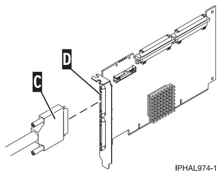
Figure 31. SCSI cable to a SCSI card
