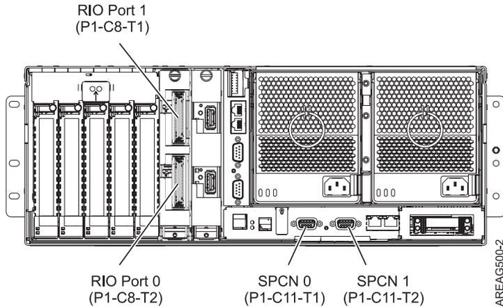
Figure 8. Model 9117-MMA connector locations
