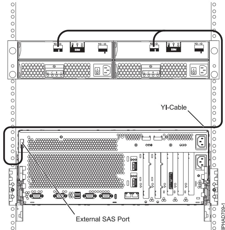
Figure 48. Single enclosure attached with YI cable to external SAS port
