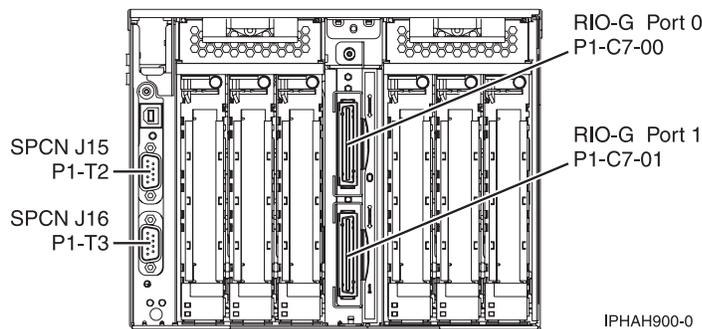
Figure 9. Model 5790 or 7311-D11 connector locations
